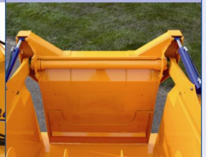
Arm reinforcement beam built into the shovel
