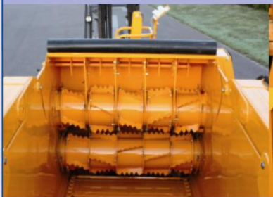
Two mechanically driven bale separators (clutch as option)
